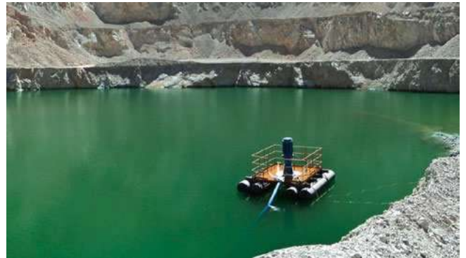
Versar Barge Pump System™ VTC (300 hp) for Mine Dewatering
