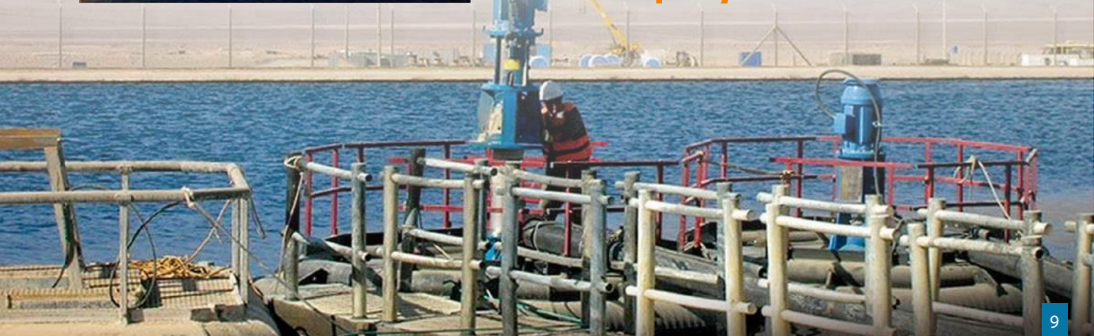
Versar Barge Pump System™ VTC 170-5E (200 hp)
